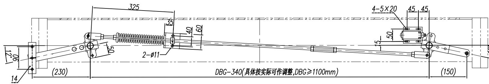
导轨面距  $DBG$  ( $DBG \geq 1100mm$ )
